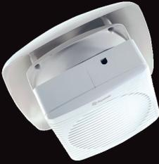
RX models are a neat way of ventilating through glazed and solid roofs and can be used vertically in windows on exposed sites such as coastal areas and high rise buildings. They are suitable for single and sealed double-glazed windows and panels up to 25mm. For flat roofs an optional roof-mounting plate allows RX models to be fitted to dressed curbs.
