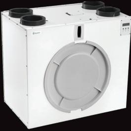
Xcell 400QVI units are designed for modern airtight buildings and are ideal for 4 – 5 bedroom houses and larger apartments. They incorporate a high efficiency heat recovery counterflow cell for heat recovery of up to a 91%, EC ultra-low energy motors and G4 filters. The three intake connection spigots located on the top of the unit make the unit ideal for locating in a loft void.
