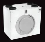
The Xcell 300QVI has been purpose-designed for modern, airtight houses with 3-4 bedrooms, or large apartments. With a counterflow heat exchanger capable of recovering up to 91% of the extracted heat, plus energy-efficient EC motors, it's a cost-effective solution. This model may be wall or loft-mounted, features a long-life G4 filter, and is Passivhaus approved.
