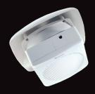
RX models are a neat way of ventilating through glazed and solid roofs and can be used vertically in windows on exposed sites such as coastal areas and high rise buildings. They are suitable for single and sealed double-glazed windows and panels up to 25mm. For flat roofs an optional roof-mounting plate allows RX models to be fitted to dressed curbs.
