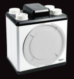
The Xcell 150QVWSB features a high-efficiency counterflow heat exchanger, providing up to 90% heat recovery efficiency. This unit is purpose-designed for modern, airtight apartments and houses, where less natural leakage can cause increased condensation and mould problems. This model has lightweight EPP construction and may be floor or wall-mounted in the loft space.
