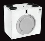
Xcell 400QVI units are designed for modern airtight buildings and are ideal for 4-5 bedroom houses and larger apartments. They incorporate a high efficiency heat recovery counterflow cell for heat recovery of up to a 91%, EC ultra-low energy motors and G4 filters. The three intake connection spigots located on the top of the unit make the unit ideal for locating in a loft void.
